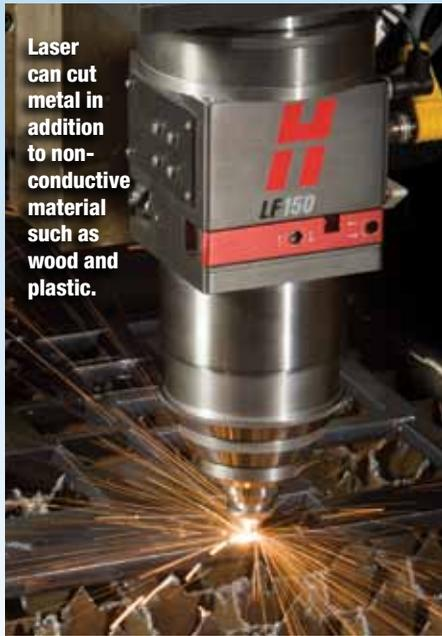
Laser can cut metal in addition to non-conductive material such as wood and plastic.
