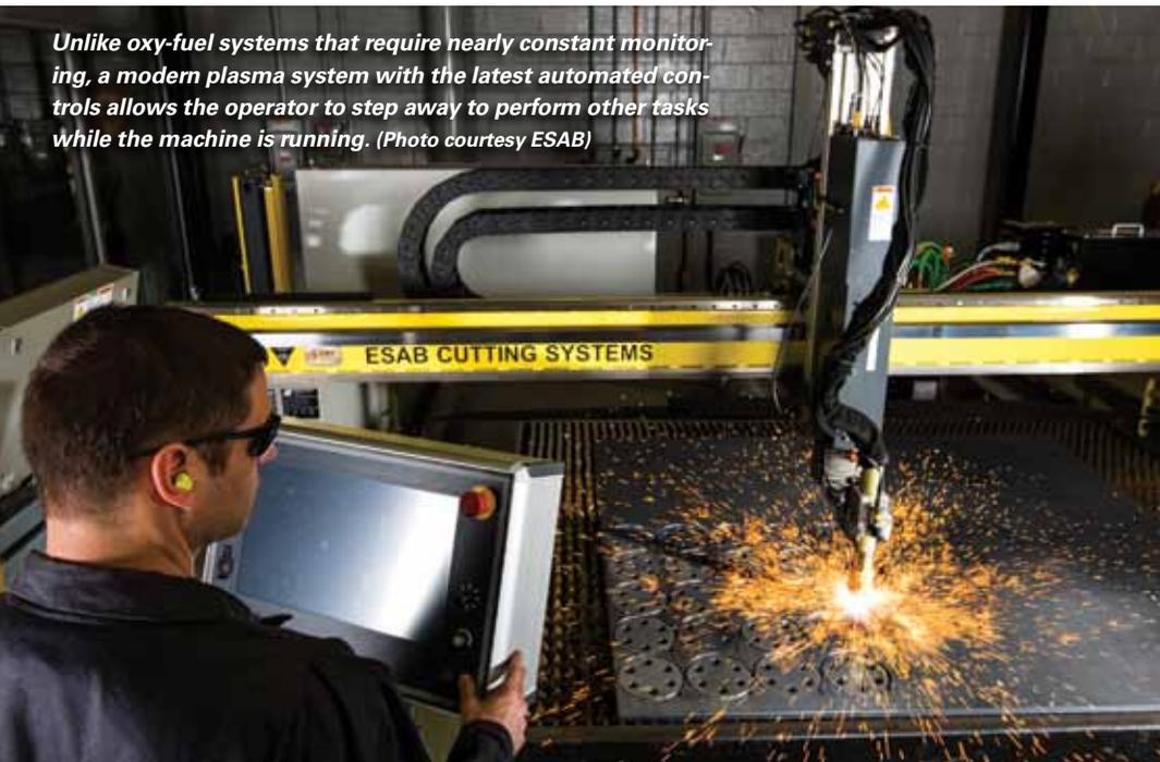
and then adjust the regulators to obtain the appropriate gas flows and pressures. While not significantly time-consuming, this manual process relied on the operator to make adjustments as the conditions changed. Automating this process ensures such adjustments are made automatically and consistently.
