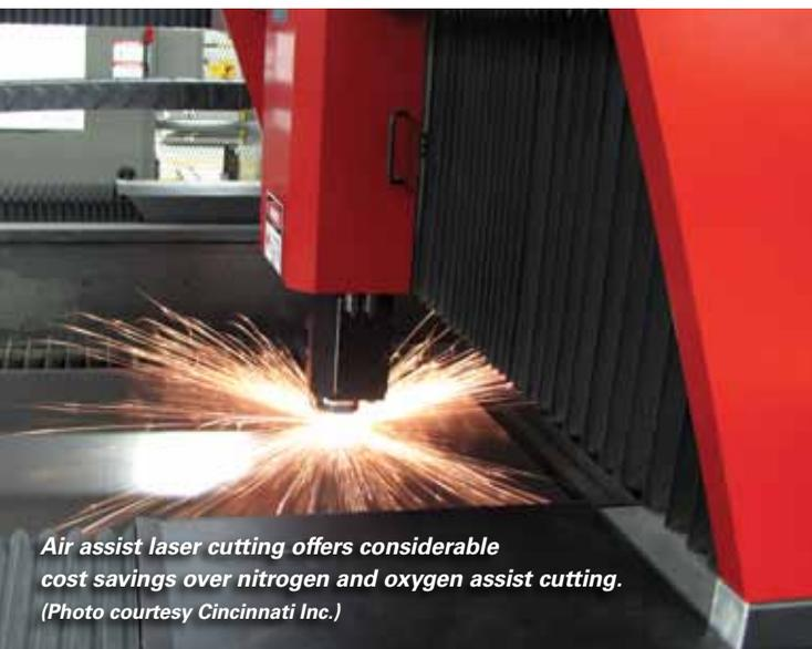
*Air assist laser cutting offers considerable cost savings over nitrogen and oxygen assist cutting.*
