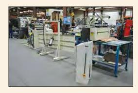
The threading table supports the material strip across the looping area for ease in thread-up of the line. In the lowered position it acts as a barrier to guard the operator from the material in the looping area.
