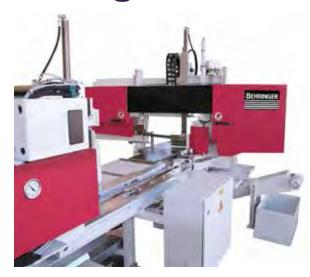
ehringer will display its HBE-320/523GA at the trade show. The fully automatic, dual-column miter saw represents the latest in sawing technology. With a ball screw servo-drive for precise control of both the saw blade and material feed, the HBE-320/523GA offers unmatched accuracy and repeatability.
